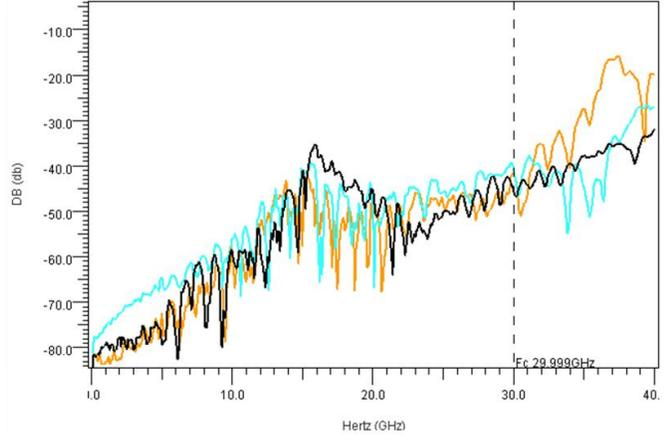
*Figure 3: Measured crosstalk for signal vias*
