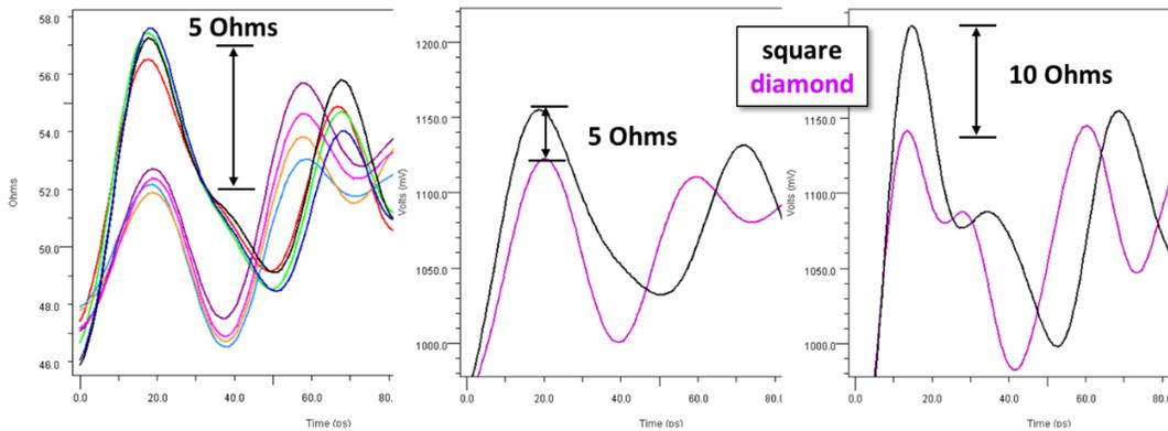
Figure 18: Single-ended TDR for stacked PCB layer model
