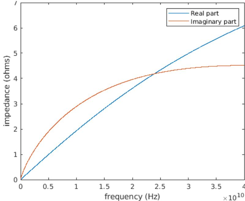
*Figure 11: Return impedance with absorbing boundary conditions*
