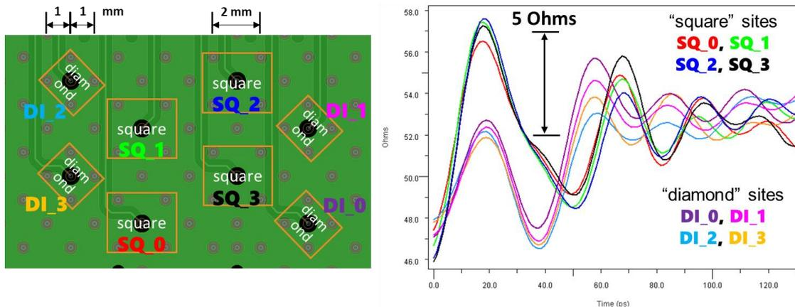
*Figure 2: Measured TDR for eight test signal vias*
