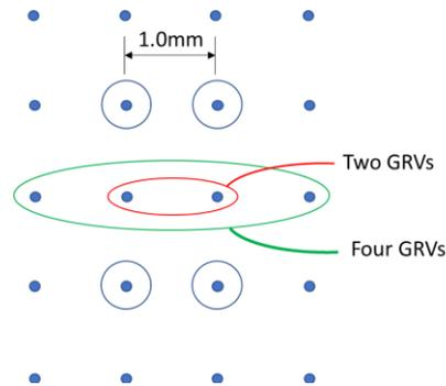
*Figure 20: Layout for differential transmission crosstalk study*
