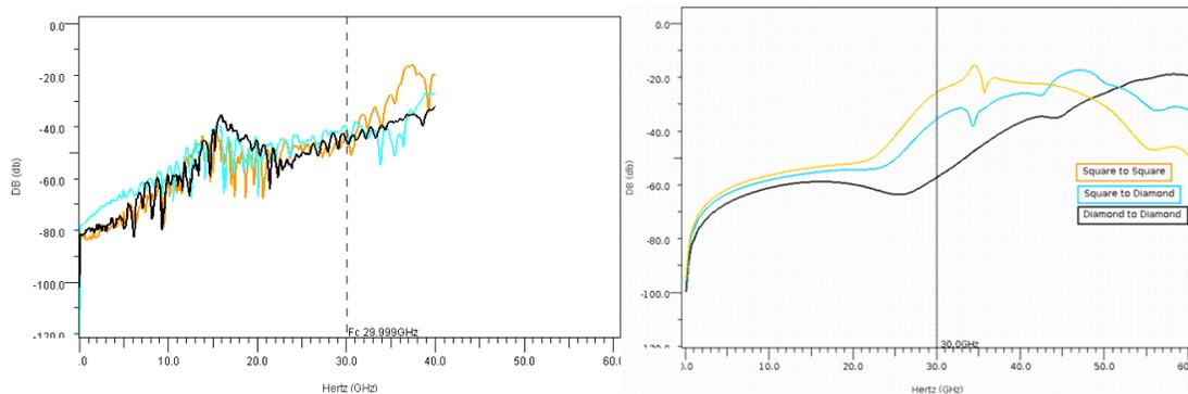
Figure 19: Measured System Crosstalk versus Via Only Crosstalk
