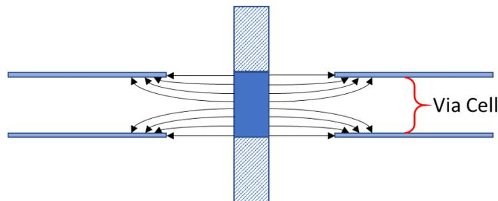
*Figure 5: Electric fields in a typical via cell*
