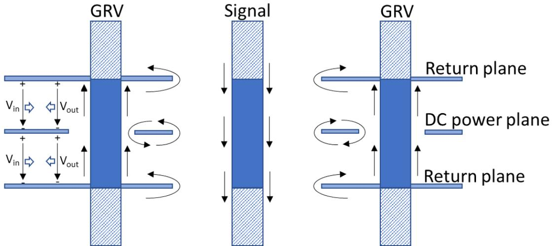
*Figure 22: Signal propagation through a DC power plane*
