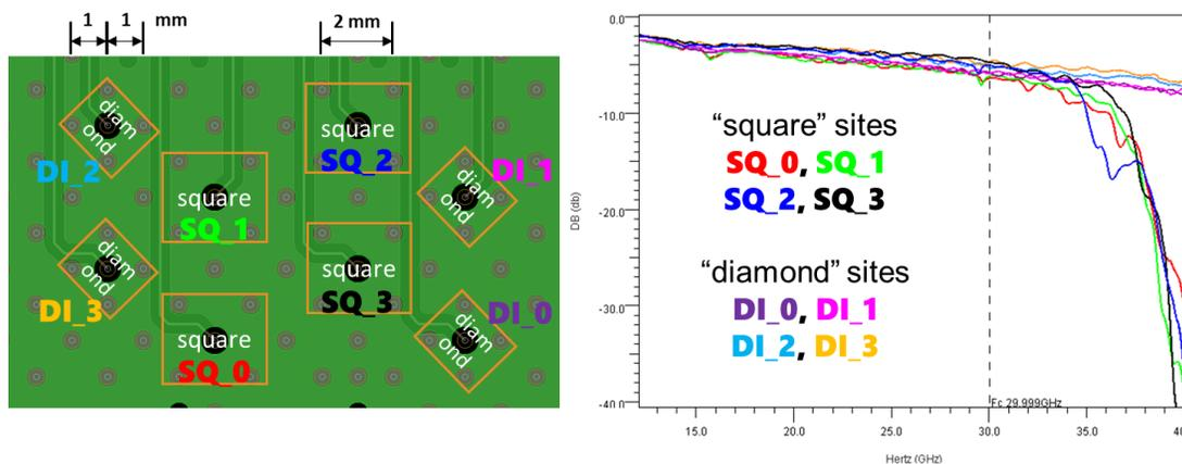
Figure 1: PCB test structure and resulting signal IL
