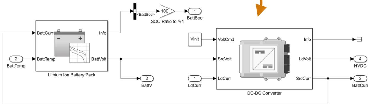
650 V Battery & DC-DC Converter
