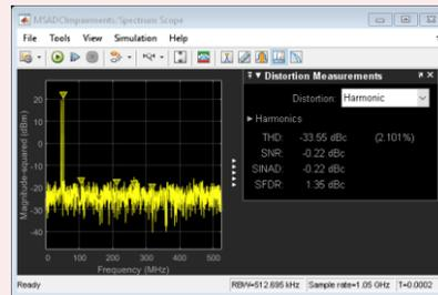
Analyze ADC with Impairments: quantization, saturation, nonlinearity, jitter
