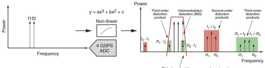
This is what happens when two tomes are input  $(f_1 \& f_2)$  into non-linear system, i.e., mixing
