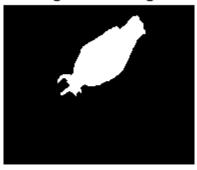
An alternate method for displaying the segmented object is to place an outline around it. The outline is created by using the bwperim function.
