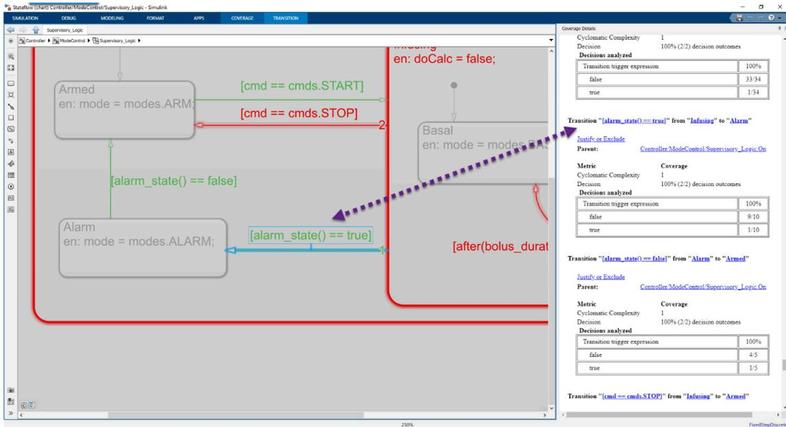
Model highlighted with coverage results. The behavior (Stateflow chart) on the left shows that the alarm was detected, and the HTML report on the right provides a summary artifact. Embedded hyperlinks provide traceability to the model under test.
