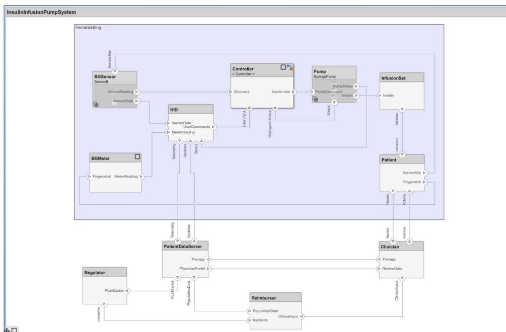
Example of system architecture in Simulink. The controller is linked to a Simulink behavior model representing a software item.
