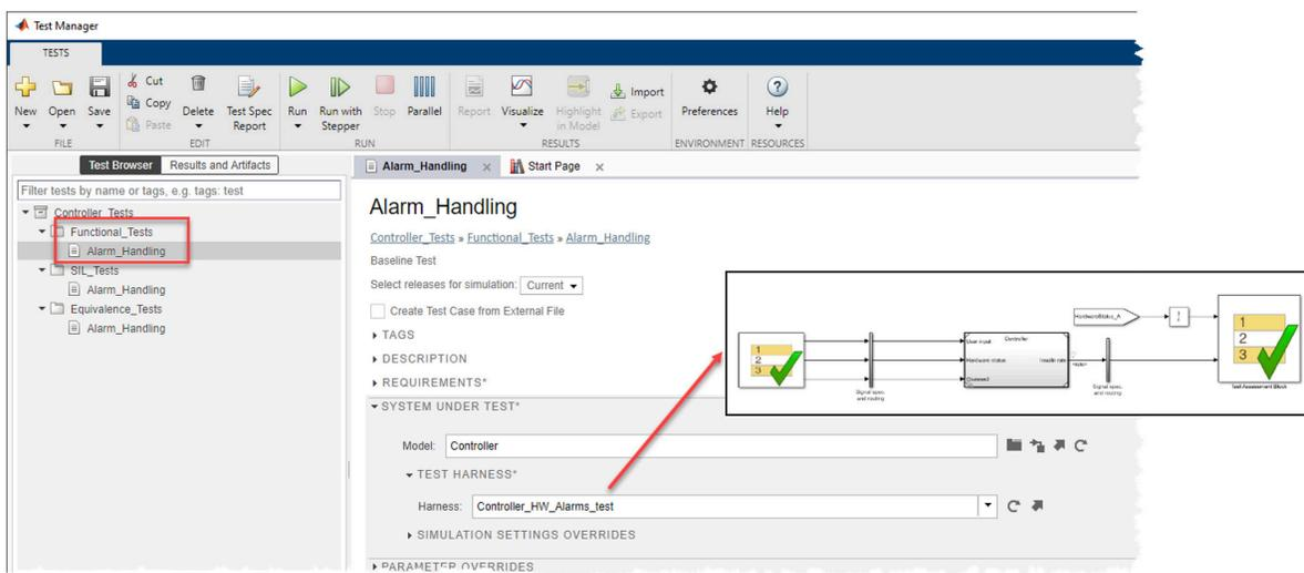
*Simulink Test implementing an alarm handling test case by calling a test harness model to exercise a design model. In the harness, the Test Sequence block provides the test vector inputs while a Test Assessment block checks the outputs.*
